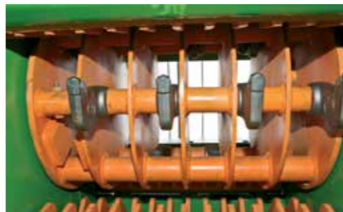
The rotor in combination with the suitable flails is the central element of every shredding system
