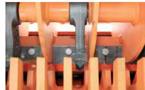
Either 18 free-swinging or 12 fixed flails are used in the Mini-Shark
