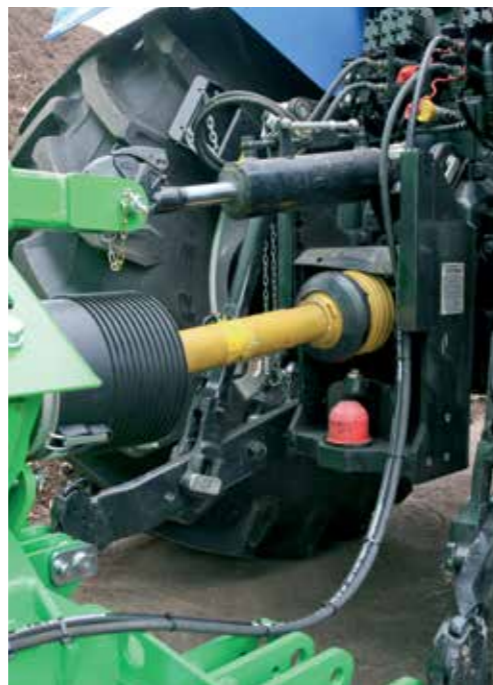
Connection by sturdy powerdrive jointed shaft with overload clutch
