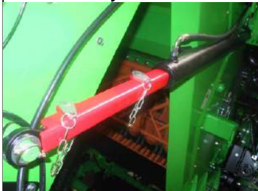
Securing of conveyors cylinder
