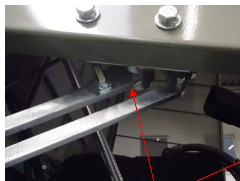
Bolt is engage in the hood securing.
