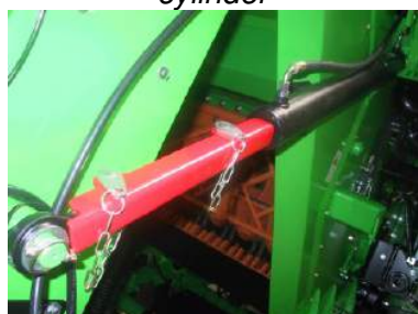
Securing of conveyors cylinder
