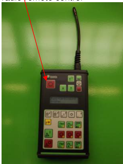
Emergency off key on the radio remote control
