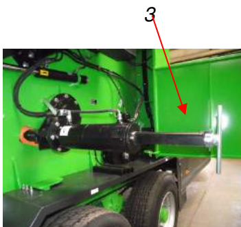
Illustration 7.15 Insert the distance sleeve
