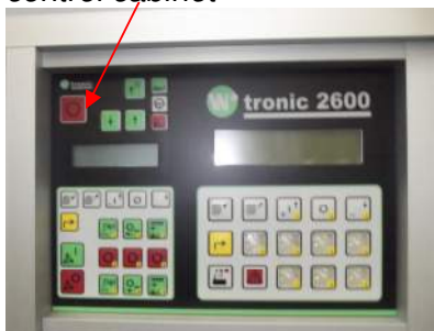
Emergency off key on the control cabinet
