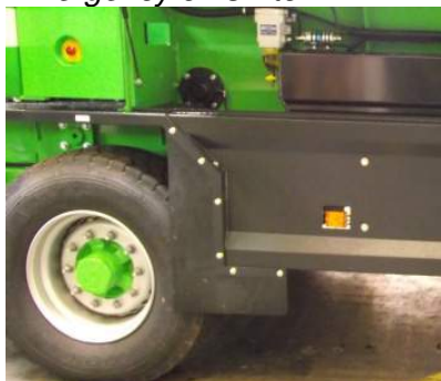
Emergency off switch
