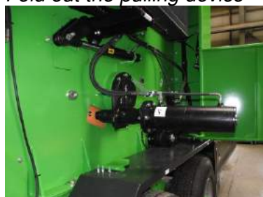
Illustration 7.13 Fold out the pulling device
