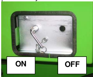
Main battery switch
