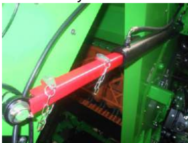
Securing of conveyors cylinder
