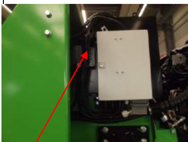
Siren is installed in the engine control bot
