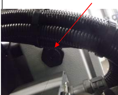
Siren is installed in the engine control bot
