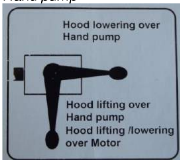
Hood lifting /lowering over Hand pump
