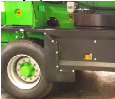
Emergency off switch
