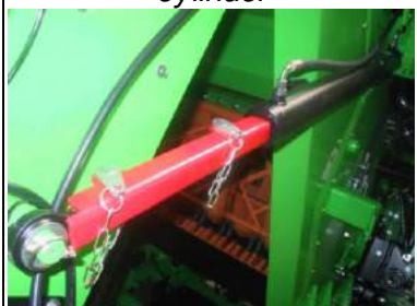
Securing of conveyors cylinder
