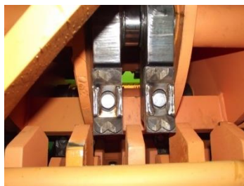
Illustration 7.18 Examine the free run of the flails
