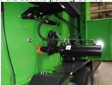
Illustration 7.13 Fold out the pulling device
