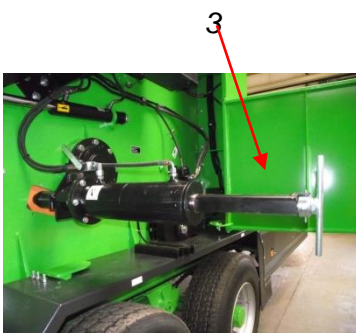
Illustration 7.15 Insert the distance sleeve
