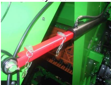
Securing of conveyors cylinder
