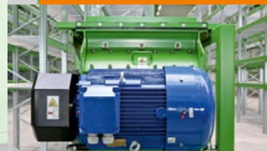
Powerful electric motor with 45 KW for throughput rates up to 30 m³/h
